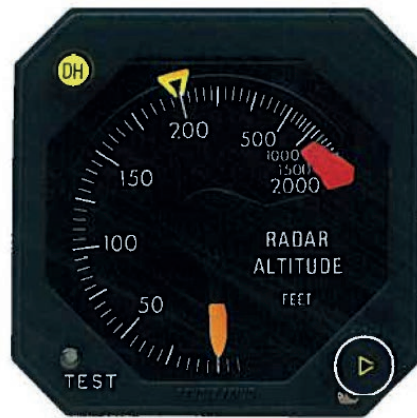
The KNI 416 Altitude Scale (helicopter presentation) gives accurate indication from -10 to +2000 feet.
