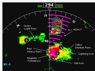
Figure 11 - IntuVue advanced hazard warnings
