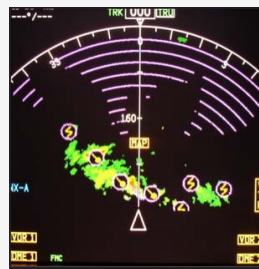
Areas of severe attenuation shown in magenta (not just at the outer edge)
