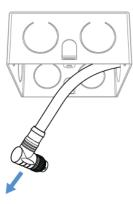
2. Pass the 4-pin male wiring harness (elbow) through the junction box, insert the 4-pin female socket at the bottom of the slave, and then tighten the nut of male plug to ensure that the male plug and female socket are locked.
