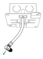
2. Pass the male plug cable harness through the junction box and the mounting floor (it is recommended to use a cable harness with a right-angle elbow male plug for ceiling installation).
