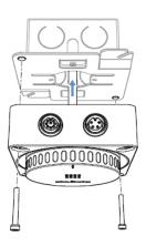
Insert the plug into the master detector and secure the detector to the mounting base plate with screws.
