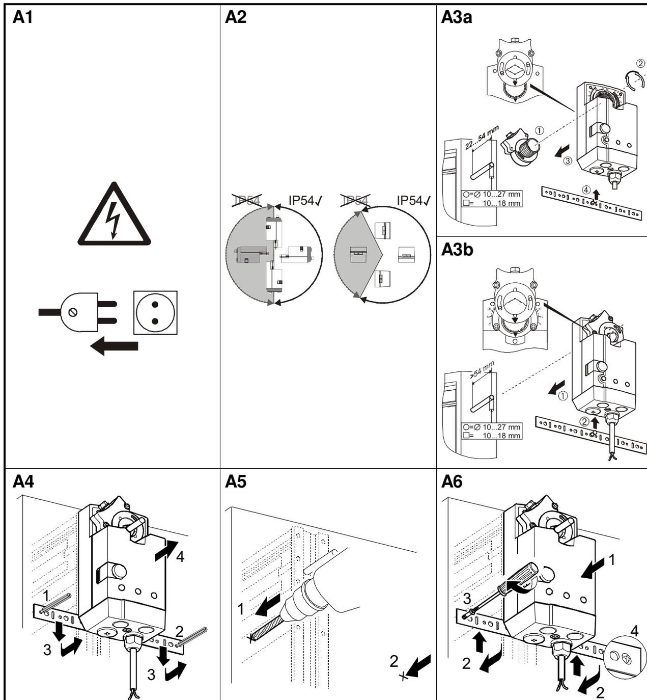
**MOUNTING ON COUNTERCLOCKWISE (CCW) OR CLOCKWISE (CW) CLOSING DAMPER**
