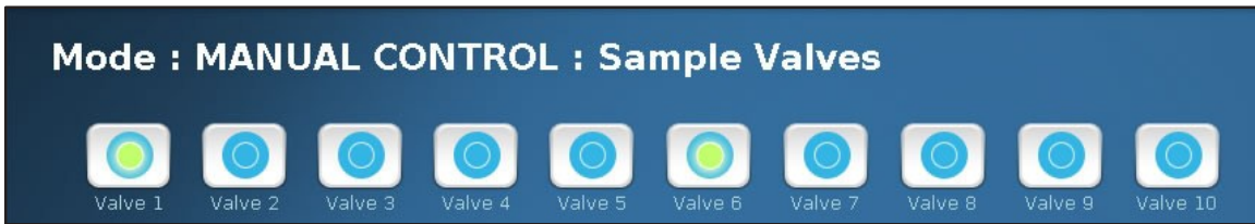
Figure 76. Sample valves manual control
